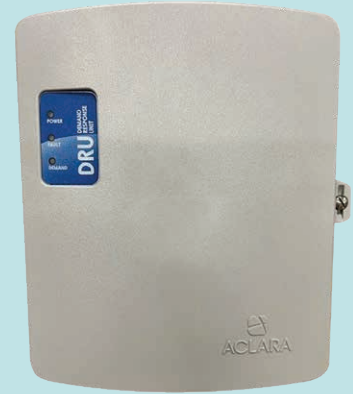
GREEN MEANS GO: You can see if the U-Shift device is turned on simply by looking for the green light. An amber light indicates we are interrupting service, and red may mean there’s an issue.
